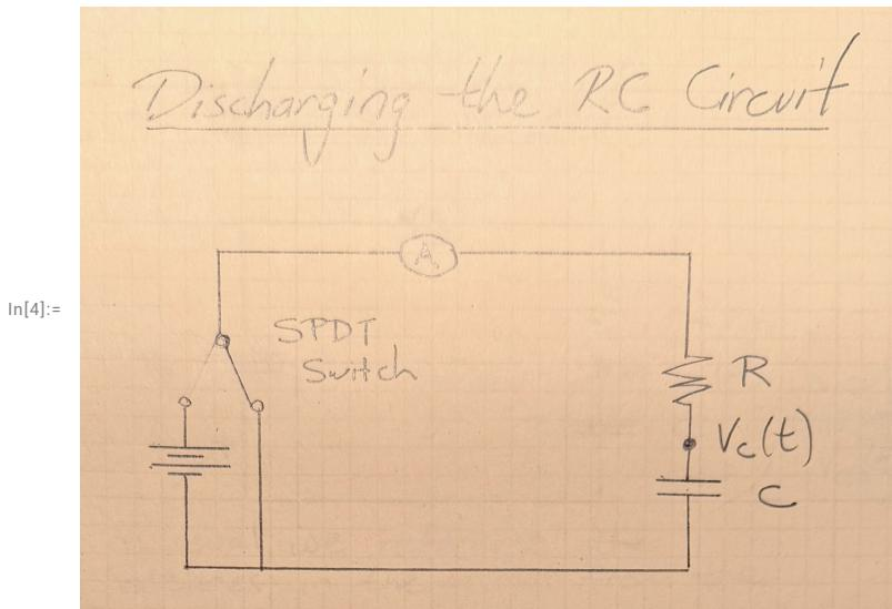
The path the current can follow now bypasses the battery, but still goes through the resistor. Because of the resistor, the current cannot discharge all at once.
