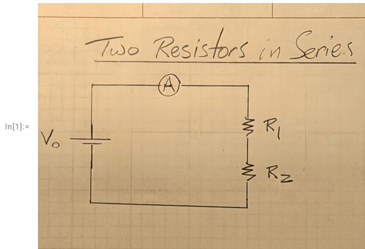
We learned that  $R_1$  and  $R_2$  connected in series act exactly like a resistor with size  $R_1 + R_2$ . What does that mean!? It means that the current through a combination of two resistors also obeys Ohm's Law, but with the constant of proportionality being  $R_1 + R_2$ .
