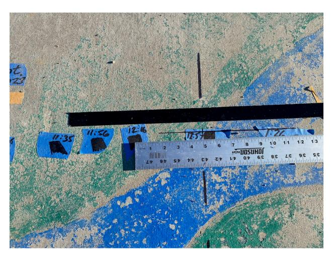
In the above photo, the shadow at 12:16pm has been placed at 0". At 5.5" is the shadow at 12:57pm. 12:57pm is 41 minutes later than 12:16pm. The North-South line is at 5". So local noon was 5.0/5.5 = 10/11 of the way from 12:16 to 12:57 or 37 minutes after 12:16 or 12:53pm.
