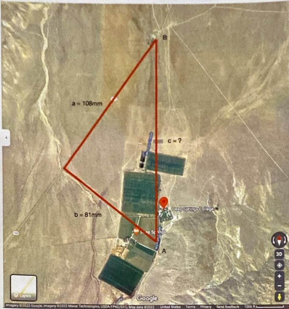
(1) Use the ordinary planar Pythagorean Theorem to get  $c$  (in mm) from  $a$  and  $b$ .  $c = 135 \text{ mm}$
