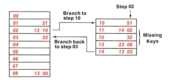
Notice in particular that the instruction originally stored in step 02 is now stored in step 10. Step 02 now contains an unconditional branch instruction to step 10. The missing keys are stored in steps 11 through 13 and the instruction stored in step 14 is an unconditional branch back to step 03 in the main program.
