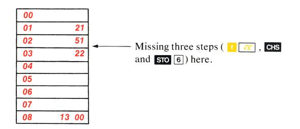
In order to add the missing steps we need to branch to one of the available program steps in program memory. The corrected program is shown below.
