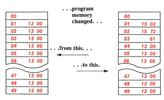
The illustration on the left shows program memory immediately after pressing **PRGM** in PRGM mode or turning the HP-25 ON. The illustration on the right shows program memory after recording the three-step example program.
