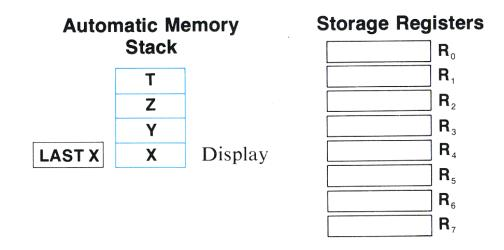
The addresses of the storage registers are indicated by number keys 0 through 7, as shown above.
