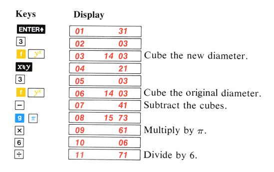
The program keystrokes for this problem are the same. Simply switch to PRGM mode **PRGM** and press **1 PRGM** to clear program memory and display step 00. Then key in the list of keys above. The keys are not executed, but are recorded in program memory steps 01 through 11. Verify that each keycode is correct as you key in each instruction by checking the displays shown.
