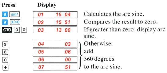
To run the program set the PRGM-RUN switch back to RUN PRGM RUN and press f PRGM so that the calculator will begin execution from step 00. Then key in positive or negative values for x. The resultant arc sine will always be positive.
