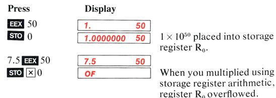
To clear a storage register overflow display, merely press CLX.
