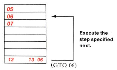
When recording an unconditional branch always follow the GIO key with two digit keys to designate the step number. For instance, to branch to step 6 the program instruction must be GIO O[6].
