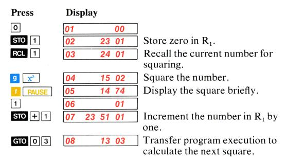
The program calculates the square of the number in storage register  $R_1$ , starting with zero. It pauses to show the answer and then increments the contents of the register by one. The unconditional branch at the end of the program is used to transfer program execution back to step 03 so that the calculation can be repeated with the new value in register  $R_1$ .
