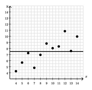
Notice that this line doesn't seem to fit the data very well. One way to measure the fit of the line is to calculate the sum of the squared residuals—this gives us an overall sense of how much prediction error a given model has.
