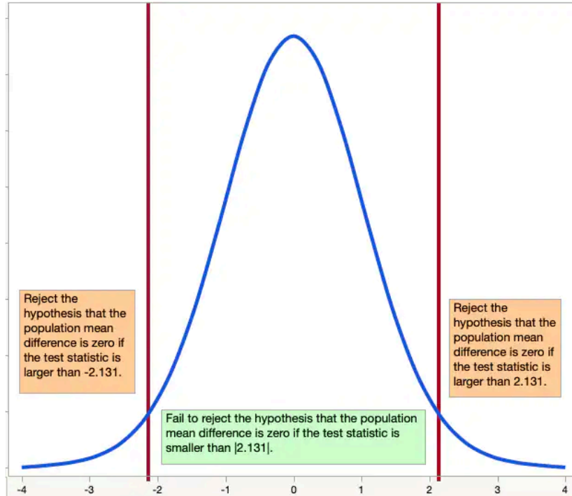
Figure 4: t -distribution with 15 degrees of freedom and \alpha = 0.05
