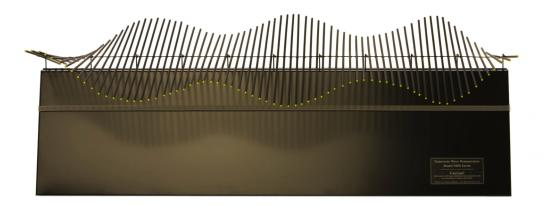
Our goal is to set up the theory so that we can simulate in Mathematica what this thing does in real life. Note that it has 72 rods. We will progress from 1 rod, to 2 rods, and then do 72 rods.
