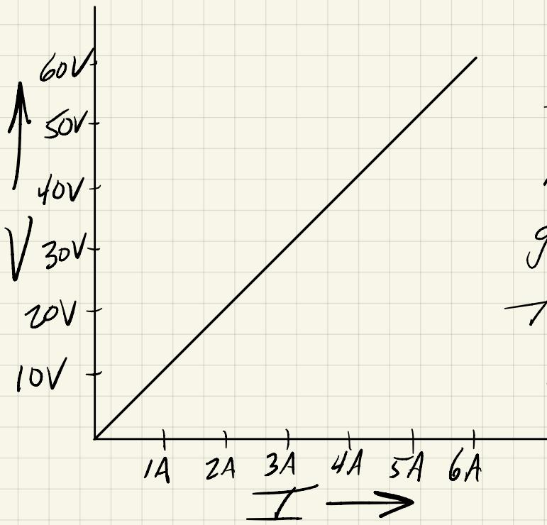
A straight line passing through the origin is the I-V graph of a resistor.
