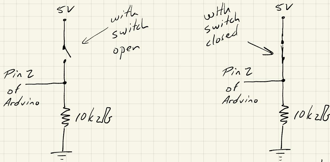
If the switch is closed, then clearly Pin 2 of the Arduino is at 5V (pin is "HIGH").
